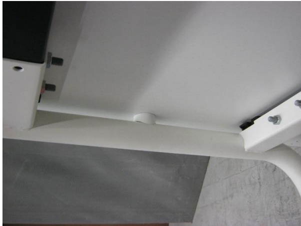
Photo 5: Tested sample 220609-7 - bottom view - detail 2 connection frame to table top and attachment of horizontal part to vertical part table leg
