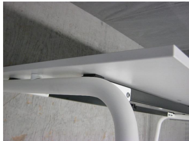
Photo 4: Tested sample 220609-7 - side view - detail 1 connection frame to table top
