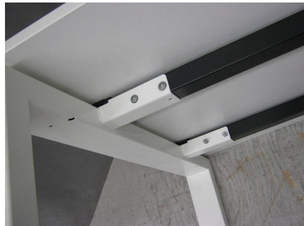
Photo 4: Tested sample 220609-5 of Techo Fount Original Leg office desk - detail connection legs to frame
