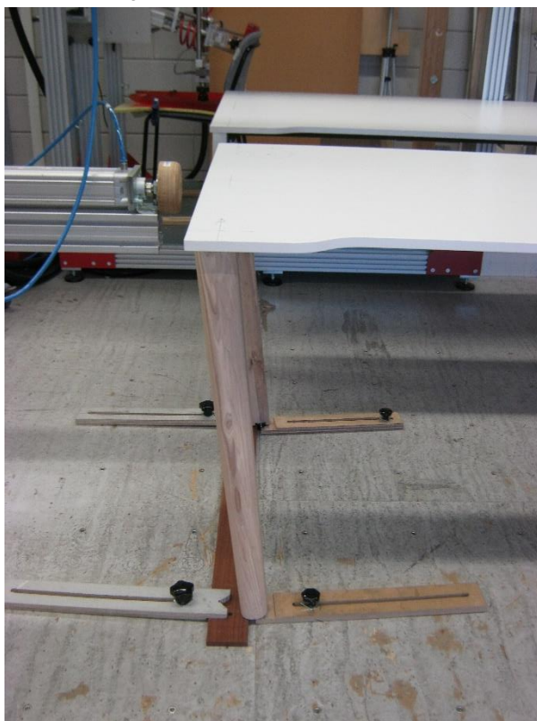
Photo 7: Tested sample 220609-1 of Techo Fount Wood Leg office desk – after horizontal static load test
