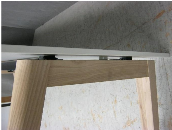
Photo 5: Tested sample 220609-1 of Techo Fount Wood Leg office desk - detail table top to legs side view
