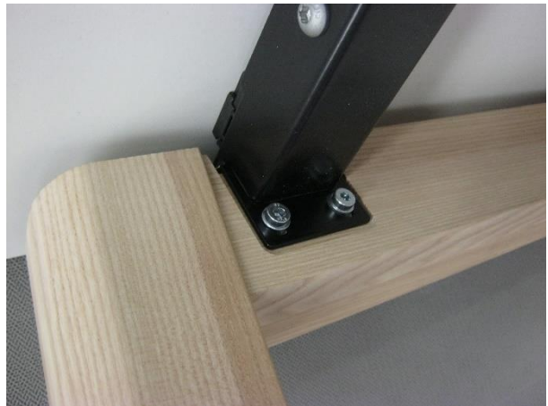
Photo 4: Tested sample 220609-1 of Techo Fount Wood Leg office desk - detail connection legs to frame
