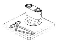
NOTE: 4mm and 5mm Hex Keys can be found under the plastic base cover.
