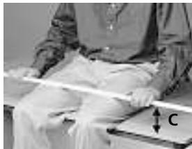
**Dimension C:** the distance between the top of the table and a ruler placed across the thighs, plus 5 cm. If this is greater than dimension B, you should use dimension C instead of dimension B.
