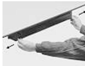
The cable dump is opened by simultaneously pulling out the knobs at the two opposite ends, on the side of the dump nearest to you. The dump will then drop open. **Caution!** If all four knobs are pulled out, the whole cable dump will come out of the suspension brackets!
